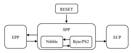
In SPP mode, software can be used to control PCR and query PSR to realize transmission of Nibble, Byte and PS/2. For specific operation steps, please refer to the IEEE1284 specification.
